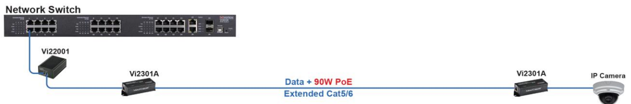
The Vi22001 can be used along with extenders to power PoE powered devices at long distances. The following chart shows how much power can be available at extended distances:
