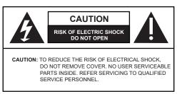
WARNING! - To reduce the risk of fire or electric shock, do not expose this apparatus to rain or moisture. This apparatus shall not be exposed to dripping or splashing and no objects filled with liquids, such as vases shall be placed on the apparatus.
