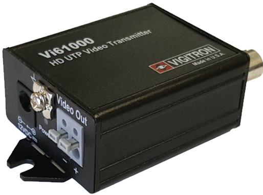
The Vigitron Vi61000 is an advanced active device that transmits HD video over unshielded twisted pair wires. It is compatible with HD-TVI, HD-CVI and AHD video formats. The Vi61000 uses Cat 5/6 UTP cables and can provide quality HD video up to 2000 feet (610 m) depending on the video format when it is paired with Vigitron Vi61001 active receiver.
