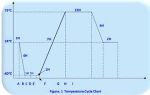
Where testing is done to known standards, those standards should be noted. The above is an example of temperature testing performed to NEMA-TS2 temperature cycle standards.
