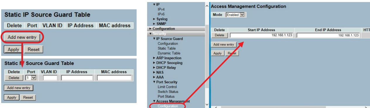
*Static IP Source Guard allows only those programmed IP access to access the individual port. Access management configuration allows access to HTTP, HTTPS, and SNMP, TELNET and SSH only from the range of programmed addresses, and rejects non-listed host access to the switch.*
