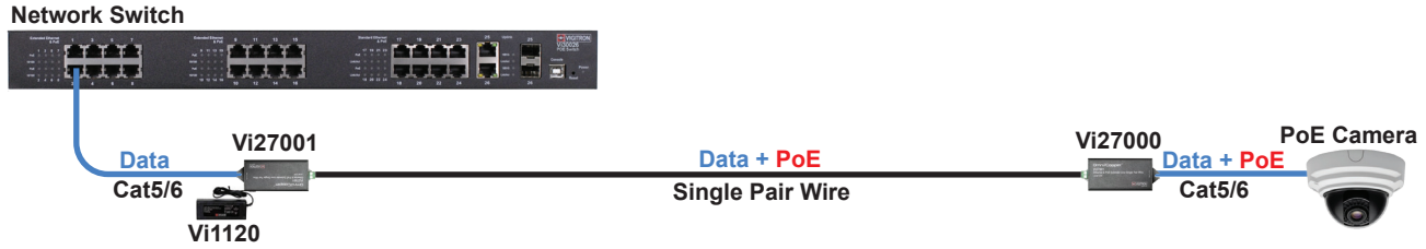
The Vi27001 receiver can use a local power supply to power Vi27000 transmitter and the IP camera using PoE.
