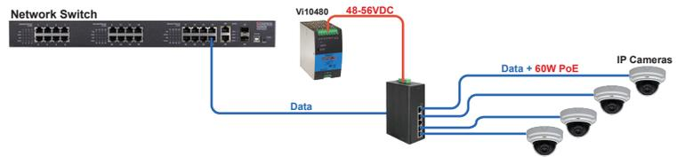
The Vi10480 can be used to power a wide variety high power PoE switches and Midspans.
